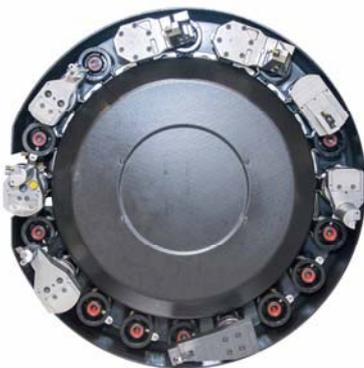
The facing heads of the machine are equipped with an HSK-A63 tool adapter. A disc revolver is integrated for the corresponding mounting tools.
