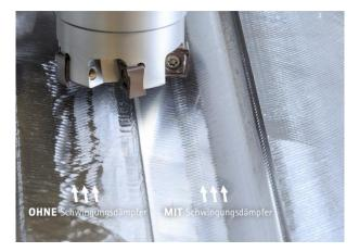
Optional vibration dampers can make a real difference: An up to 50 percent increased material removal rate and up to 60 better surface finishes.
