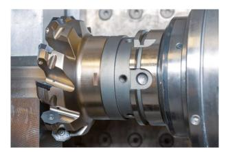
The NeoMill-8-Face face milling cutter with its inserts with eight cutting edges is the first choice for machining steel and stainless materials. The face milling cutter MAPAL Präzisionswerkzeuge Dr. Kress KG
