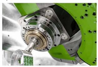
The horizontal machining centre, the 3-axis milling head and the ISO shoulder milling cutter SPM-Rough achieve best results when used together.
