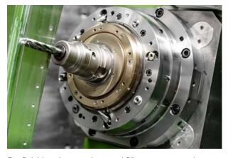
For finishing deep pockets and filigree structures in one go, Zimmermann relies on the solid carbide milling cutter SPM-Finish.
