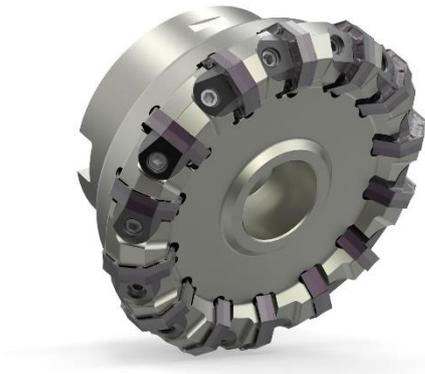
The face milling cutter NeoMill-16-Face is equipped with indexable inserts with 16 cutting edges and machines the connecting surfaces for the manifold flange and exhaust flange. ©MAPAL
