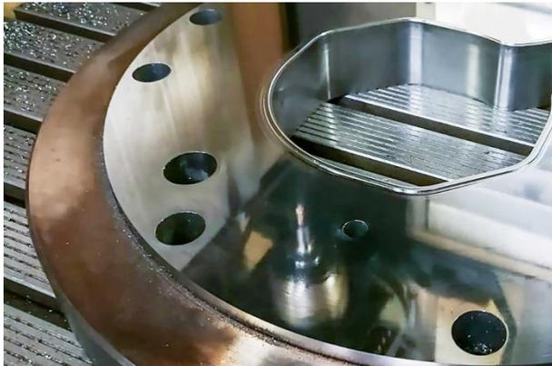
Brilliant result without grinding: to re-set a broken-out ring tooth of a large part made of hardened tool steel, HaGeForm created a perfect surface by roughing with the OptiMill-3D-HF-Hardened and finishing with the OptiMill-3D-HF-Hardened. The ring tine was finished with an OptiMill-3D-CR-Hardened. ©MAPAL
