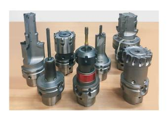
CastAlum mainly uses PCD tools from MAPAL for drilling and milling.
