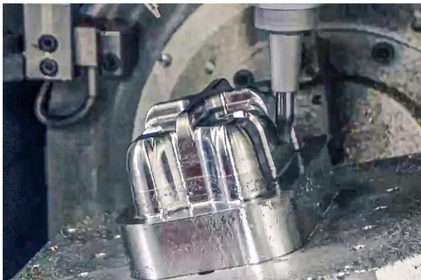
Thanks to its special geometry, the OptiMill-3D-CS shoulder radius milling cutter can be used for 5-axis finishes of workpiece sides with a high material removal rate, which reduces machining time. ©MAPAL
