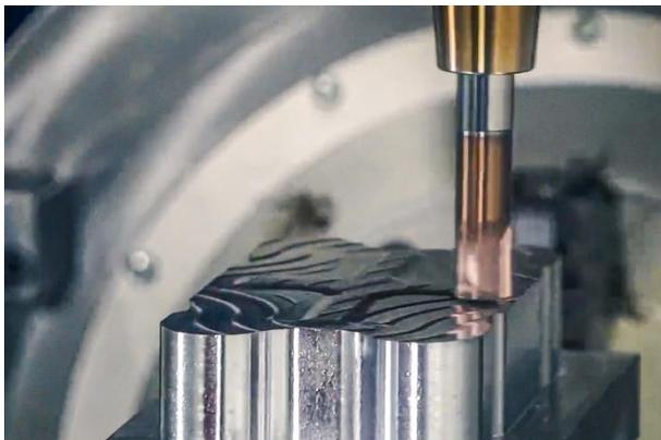
The high-feed milling cutter OptiMill-3D-HF-Hardened is used for high-precision roughing of large amounts of material. ©MAPAL
