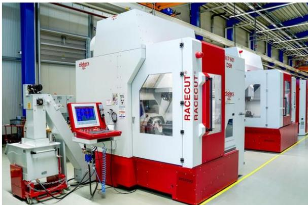
The Rödgers RXP 601 DSH 5-axis HSC milling machine, designed for highest accuracy requirements and high metal removal rates. ©Rödgers
