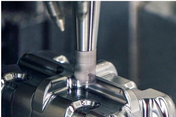
The NeoMill-3D-Finish radial indexable insert milling cutter is universally applicable for finishing all kinds of workpiece materials and machining situations. ©MAPAL
