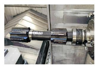
The multi-stage tool developed by MAPAL for this application has a total of three indexable inserts and 15 guide pads. ©MAPAL
