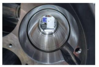
The bores have three different diameters and must be machined with high precision. ©MAPAL
