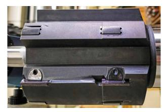
In the front area, the tool has two indexable inserts for the diameters 99 and 98 mm. Both inserts can be set radially and at an angle to the longitudinal axis. ©MAPAL
