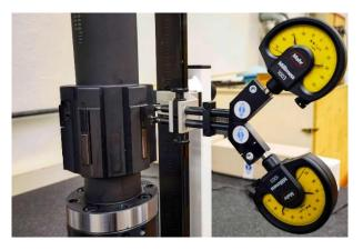
The setting fixture enables the radial position and angle of the inserts to the direction of the longitudinal axis to be checked and set using highly accurate dial gauges. ©MAPAL
