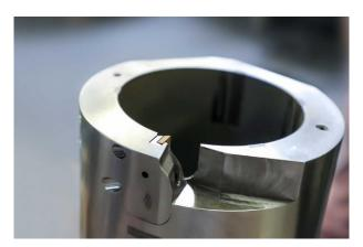
MAPAL's EasyAdjust system reduces the setting times for highprecision reaming tools. The back taper is integrated in a cassette, meaning that no manual adjustment is necessary.
