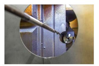
In order to reduce the weight, a relief bore is drilled into crankshafts.
