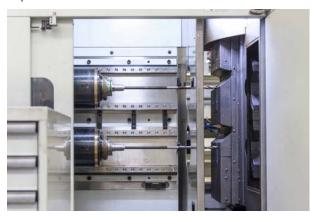
The tool holder of the long drill alone is 480 mm long when machining the crankshaft for a 6-cylinder engine.
