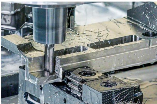
The OptiMill-Tro-Titan finishes the pocket wall. The complete depth is machined in one cut. ©MAPAL
