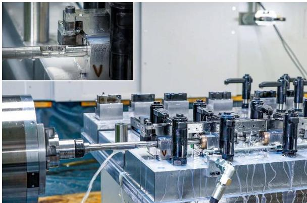
The line boring bar with a diameter of 17 mm and total length of 685 mm finishes the machining of the main bore. ©MAPAL
