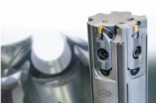
The detailed view of the fine boring tool shows the three asymmetrically arranged indexable inserts. The part can be seen in the background.
