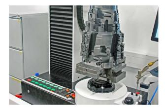
The fine boring multi-stage tool with 20 steps supplied by MAPAL is equipped with 58 PCD cutting edge and 22 PCD guide pads.
