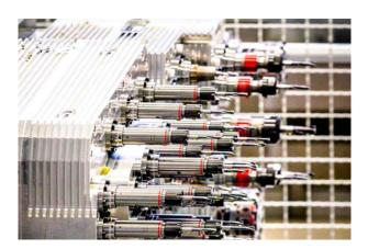
Complex multi-spindle machining head for the simultaneous machining of bores and fittings in a single machining step. Photo provided by GRÜNER
