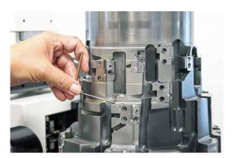
The cutting edges can be finely adjusted in various directions by means of numerous adjusting screws.
