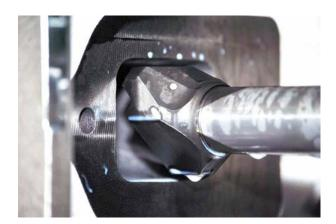
Process-reliable machining with the customer-specific face milling cutter with ISO indexable inserts from MAPAL.
