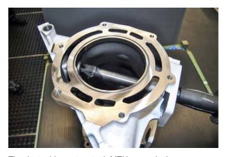
Thanks to this custom tool, MTU exceeds the evenness specifications by a factor of 10. The milling head is mounted at a suitable angle to the tool adapter. This allows it to be retracted without being turned and in this way saves time.
