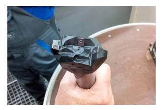
MAPAL develops a special face milling cutter for finish machining. Its four lengthadjustable, asymmetrically arranged indexable inserts allow face milling of the mounting surface by only going over it partially.
