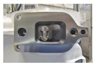
... the exhaust gas guide systems made of heat-resistant sheet metal are fixed with two screws per cylinder.
