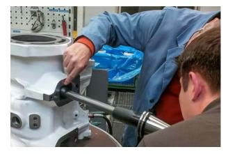
The approx. 70 x 35 mm mounting surface can only be machined through the rectangular inlet opening opposite at a distance of approx. 300 mm.
