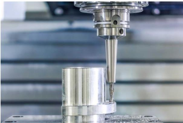
Due to the geometrical freedom of additive manufacturing, the use of hydraulic chucks is possible even with large tool restrictions.
