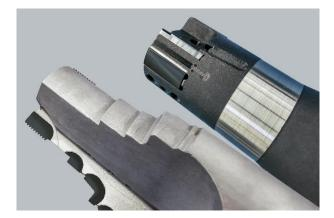
The PCD multi-stage tool (left) is used to pre-machine the calotte among other things, and to drill out and circularly mill the fine thread. The fine boring tool with
