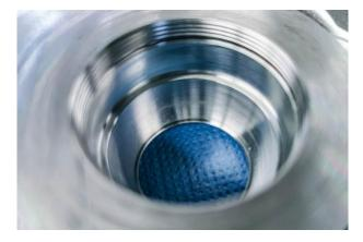
Close tolerances of up to  $\pm$  5  $\mu m$  must be maintained when machining the dome bearing. Extremely tight tolerance specifications also apply to the fine thread.
