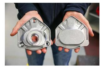
Forged aluminium strut mounts for connecting the spring strut rod end of a vehicle axle to the chassis.
