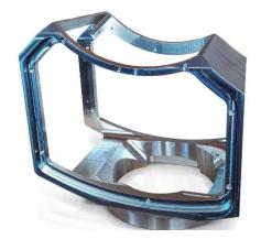
Component made of the high-strength aluminium alloy 7075 for the C-axis of a laser with a machining rate of more than 80 percent The filigree geometry required a lot of care in planning the stresses and the milling strategy. (picture: Bonertz Technik GmbH)
