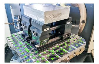
HPB machine tables from Bonertz Technik GmbH can usefully replace the outdated T-slot standard and are used wherever zero-point clamping systems are too inflexible. The interplay of vertical and horizontal grooves simplifies alignment.
