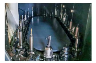
The view into the tool store of one of the milling machining centres shows various MAPAL tools.
