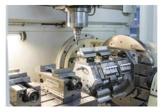
In addition to the switch from carbide tools from various manufacturers to PCD tools from MAPAL, the use of a tower with 24 clamping positions significantly increased throughput and process reliability.
