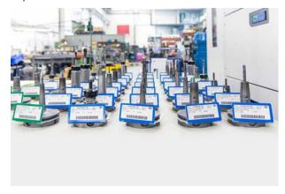
Prepared tools waiting to be used in the machine. Clearly identifiable via a barcode. Walter Formenbau purchases 80 per cent of its tools and chucks from MAPAL.
