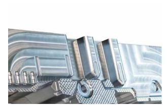
Complex clearance surfaces characterise the moulds at Walter Formenbau. Here using the example of a mould for a battery tray of an electric vehicle.
