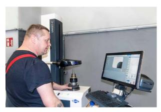
On the UNISET-C tool setting device, David Frommhold prepares the tool system for production use. He receives the measuring program directly from the CAM system. The measurement protocol is transferred to the machine via c-Com and the c-Connect Box.
