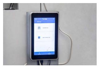
A c-Connect Box is connected to two machines at Walter. This is used to transfer the measurement data from the tools to the machine.
