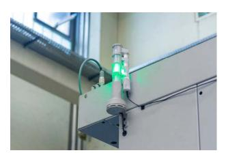
Walter uses another advantage of the c-Connect Box – the status of the machine traffic lights is monitored via sensors.
