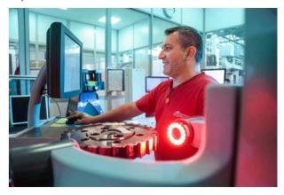
An employee measures a special disc milling cutter from MAPAL in the configuration area. Bildquelle: Hitachi Automotive Systems Group
