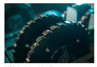
MAPAL has designed disc milling cutters as custom tools in order to best fulfil the machining tasks at Hitachi Automotive Systems. Bildquelle: Hitachi Automotive Systems Group
